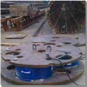
Three 6000 kip O-cells Assembled with Plates
