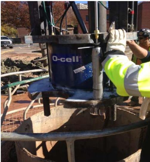
Fugro Loadtest was employed to provide foundation testing experience and equipment to Seaboard Foundations, Inc. in order to optimize the design parameters for foundations of the new building. Full scale O-cell load testing was performed prior to the ground breaking ceremony on a 29 m deep bored pile. Construction of the pile included multiple casings in the overburden soils and a 2 m long socket into bedrock.
